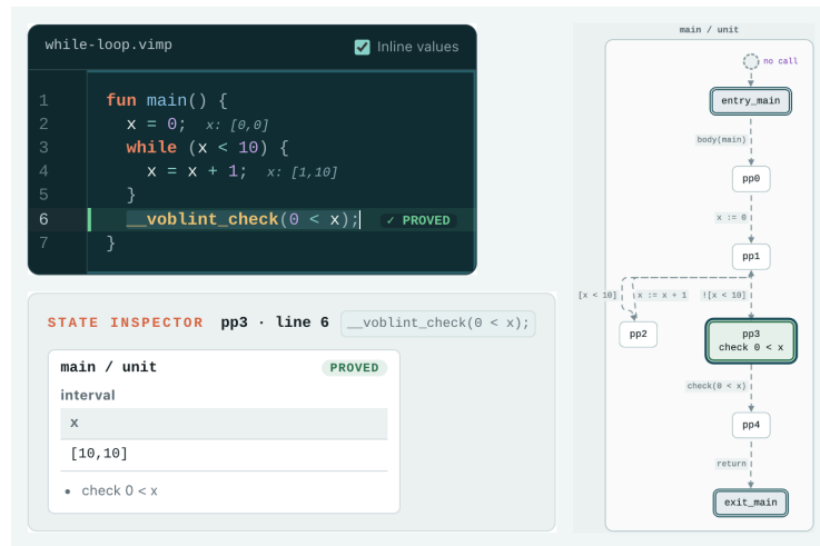
(a) one run in three views: the check's verdict in the editor, the state inspector at the check, and the solved graph. Settings analysis interval, globals warrow, context none open this run .
